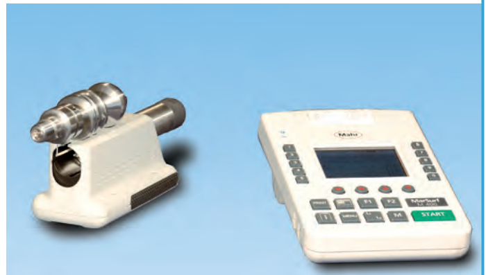
Upside down measurement with vee-block Automatic zero setting of the BFW-250
